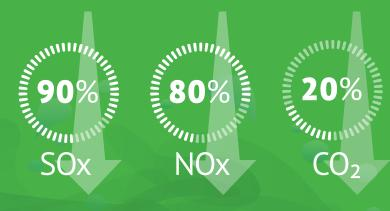
LNG reduces emissions significantly, including a 90% reduction in sulfur oxide (SOx) and particulate matter; a 80% reduction in nitrogen oxide; and a reduction of carbon dioxide (CO<sub>2</sub>) of more than 20% per container, compared with fossil fuels generally used in the international maritime industry.
